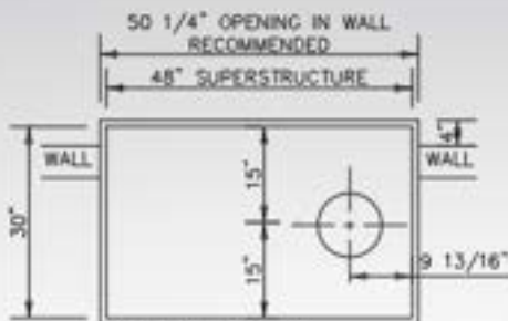
10"Ø EXHAUST DUCT STUB 84" A.F.F. FHD-1362
